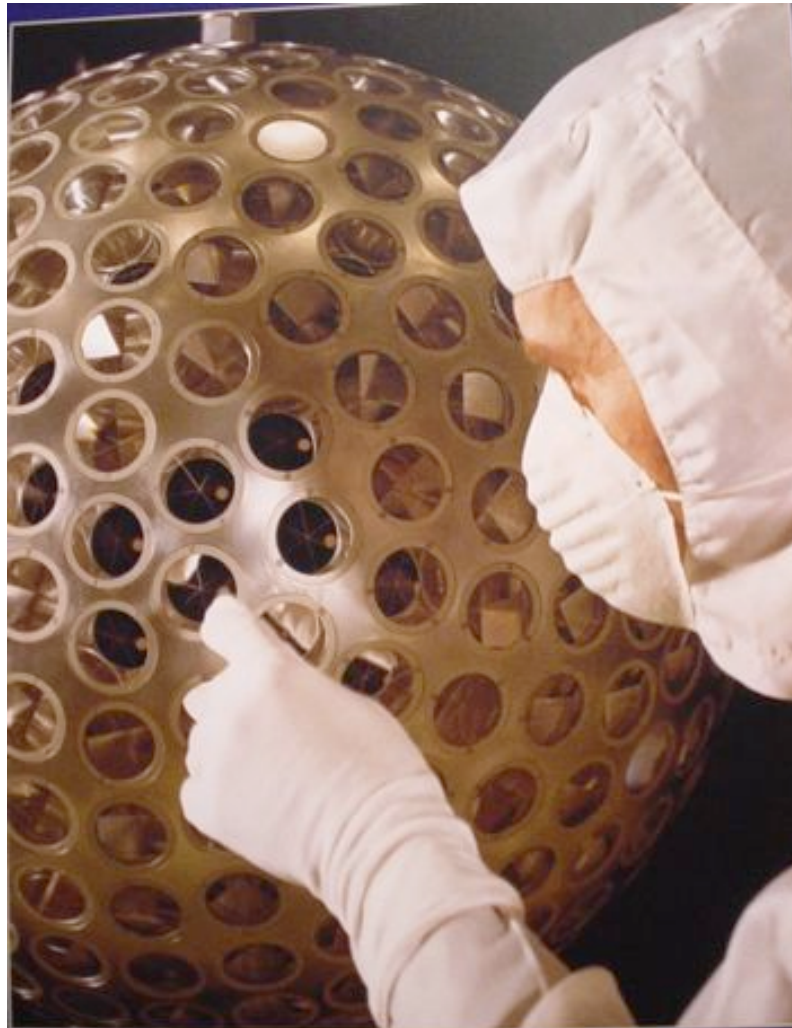
Laser Geodynamic Satellite Experiment (LAGEOS) LAGEOS satellites reflect laser beams transmitted from ground stations back to sensors on Earth. The first
